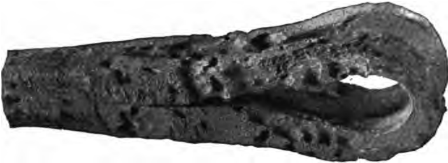
FIG. 8.—A Corroded Brace.
